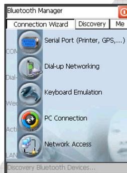
3. Tap on the "Me" button to enter the related window; then, tap on the "ON" button to activate the Bluetooth® module. The module activation may be also performed by using the WIRELESS COMMUNICATION applet as described in par. **Errore. L'origine riferimento non è stata trovata.**
