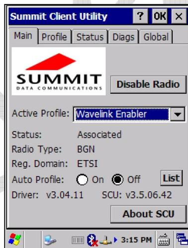
The *Active Profile* window displays the current profile and lets user to change it. The *Disable Radio* button turns off the radio card; after deactivation the same button changes to *Enable Radio* so the radio can be reactivated. To close the application, press the close button at upper-right corner of window.
