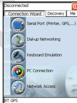
The “Serial Port” button starts communication through the Bluetooth® serial port COM 5 (typically used for connection with GPS devices).
