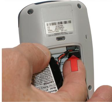
4. For correct locking, first insert the upper part of the battery cover, then the lower and screw the two screws placed on the back bottom.
