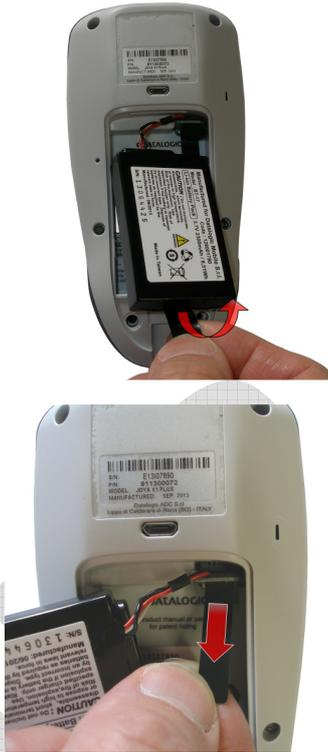
3. Install the new battery pack, first insert the connector respecting the right way, then the upper side, finally the bottom side, leaving the plastic strip available for future replace.
