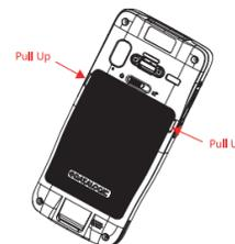
4. Open the battery cover and take out the battery in the direction shown
