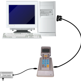
Figure 17 - Downloading Data with F734-E
