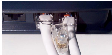
Figure 12 - Linking the cable shields
