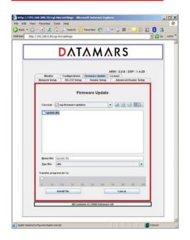
The GUI-version running on the browser offers the user a tool to update the software of the "R-IN 1300 Reader".
