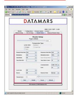
The "ReaderSetup" tab allows users to specify overall properties of the reader. It is possible to specify: the antenna power: 0 mW - 4 000 mW (1000 mW = 1 W; 2000 mW = 2 W; etc. ) the technologies of the transponders being used: ISO-15693 I-Code I the ISO-15693 properties (see corresponding ISO-specification) Request/Response Data Rate Modulation Type/ Modulation Index Quiet Mode /Quiet Storage Time Slots
