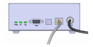
A direct Ethernet connection between a PC and "R-IN 1300 MID" reader is also possible, with an *Ethernet Cross Cable* (supplied together with the reader). Refer to Appendix A for more details on how to do this.
