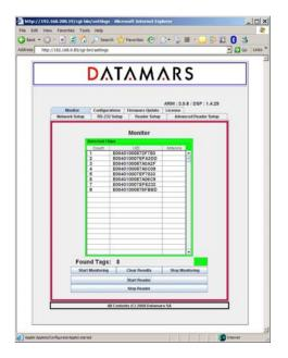
The monitor tab is used for verifying whether the reader is active or not.
