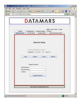
The "Network Setup" tab allows users to specify whether the reader has a fixed IP-Address (in this case the ip-address and port must be specified) or a dynamic one (DHCP) *not available yet*. After having changed the IP-Address, the browser must be closed and a new login must be done using the new IP-Address of the reader.
