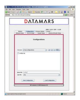
The "R-IN 1300 Reader" offers a tool giving the user the possibility to save and/or reload configuration files.
