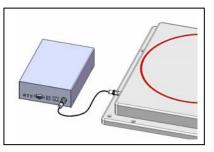
**Δ** You can not use cable other than the 3.5m coaxial 50Ω cable supplied by **Datamars.** Additional extension cables at disposal.
