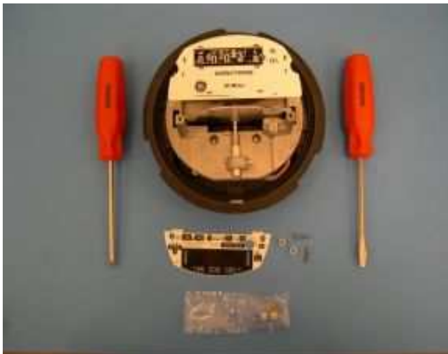
GE 2 - .25 Nylon Spacers 2 - 4-48X1/2" pan head screws
