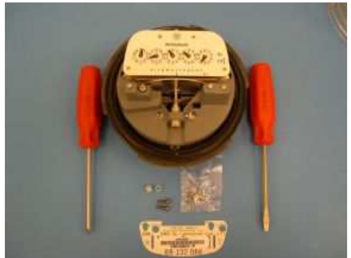
Sangamo 2 - .25 Nylon Spacers 2 - 5-40X 1/2" screws
