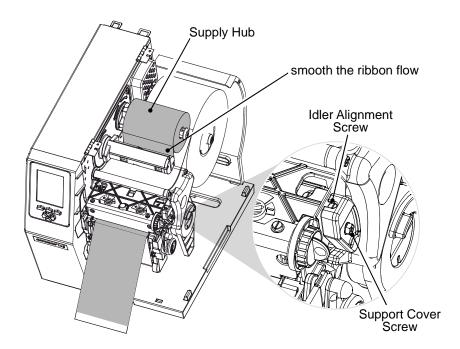
E) Wrap the Ribbon in a clockwise direction around the Take-Up Hub. Press the TEST Button on the Front Panel then use the UP / DOWN Buttons to select the RIBBON TEST LABEL. Select a small quantity of labels and press the ENTER Key. As the labels are output, observe the flow of the Ribbon from the Printhead Assembly to the Take-Up Hub. Proceed according to your observations:
