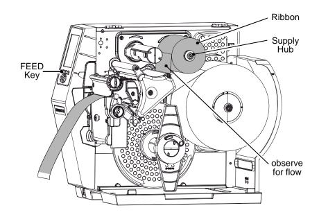
D) Slightly loosen the Support Cover Screw and, while repeatedly pressing the FEED Key, slowly adjust the Idler Adjustment Screw to smooth the ribbon flow from the Supply Hub. Afterward, carefully tighten the Support Cover Screw, and then feed several more labels to verify your adjustment.
