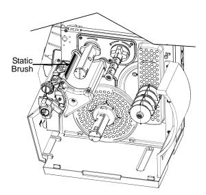
**Note:** The Static brush should be installed so the bristles are as close to the ribbon without actually touching. It may be necessary to install a roll of ribbon in order to properly align the brush to the ribbon.
