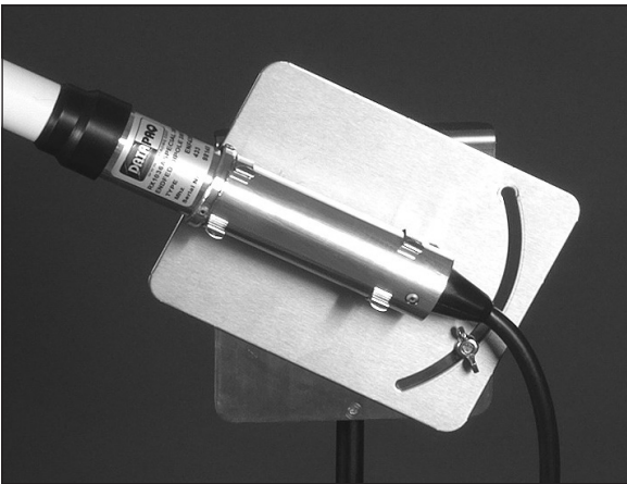
Correct fitting of unity-gain end-feed antenna in the rotating clamp of its antenna stand.
