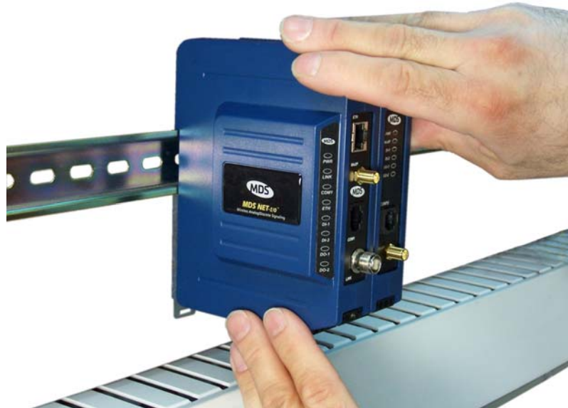
Figure 1-6. Mounting NETio Equipment to DIN Rail (Hook unit over top of rail, and push in at bottom)
