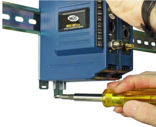
Figure 1-7. Removal of NETio Equipment from DIN Rail (Pull down on tab and swing bottom of unit away from rail)
