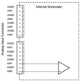
Figure 18 Equivalent Circuit for Differential Analog Inputs Connector
