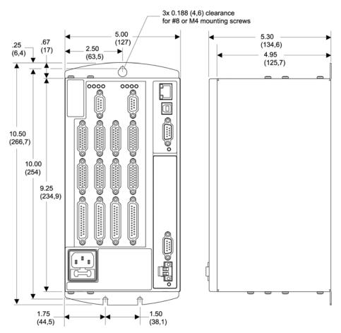
Figure 23 Mounting Specifications for ACR9000 and ACR9030 6/8 Axis Configuration
