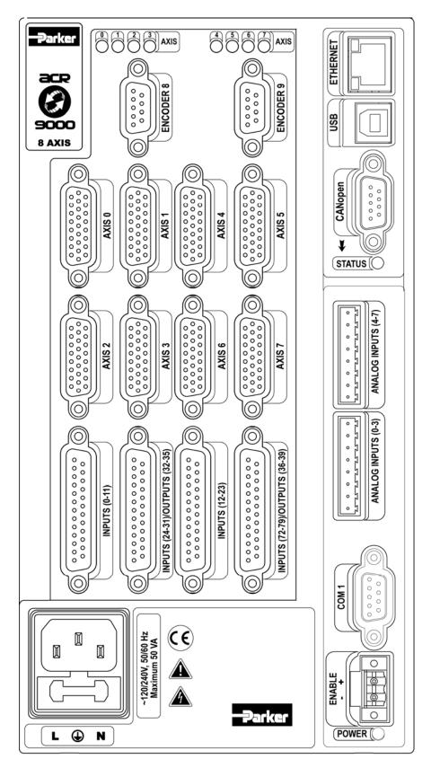
Figure 5 ACR9000 Stand-Alone Controller 6/8 Axis Front Panel Interfaces
