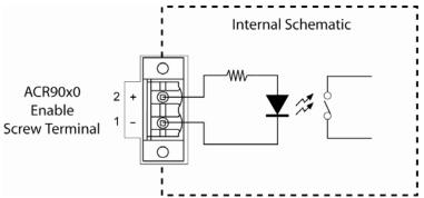
Figure 17 Equivalent Circuit for Motion Enable Connector
