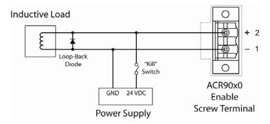
Figure 27 Loop-Back Diode with Shared Power Supply
