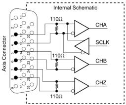
Figure 14. Equivalent Circuit for Encoder
