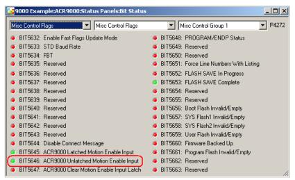
Figure 32 Motion Enable Input Fault
