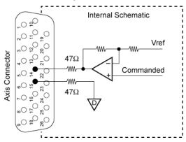
Figure 10 Equivalent Circuit for Drive AOUT Outputs
