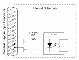
Figure 15 Equivalent Circuit for GP Inputs/Trigger Inputs Connector
