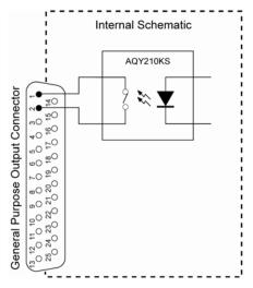
Figure 16 Equivalent Circuit for Outputs
