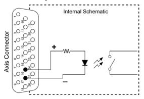
Figure 11 Equivalent Circuit for Drive Fault Inputs
