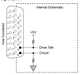
Figure 13 Equivalent Circuit for Drive Talk Signals
