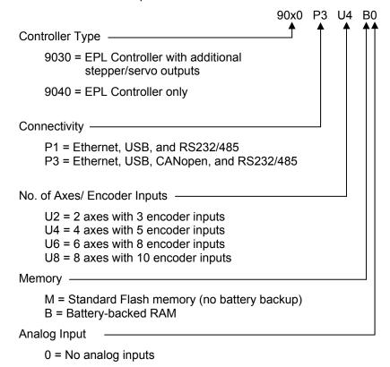
9030P1U6B0 = ACR9030 with COM port, Ethernet, and USB, 6 axes with 8 encoder inputs with EPL, battery-backed RAM
