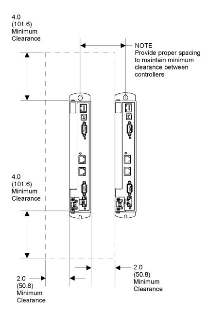
Figure 26 Mounting Clearance for ACR9040
