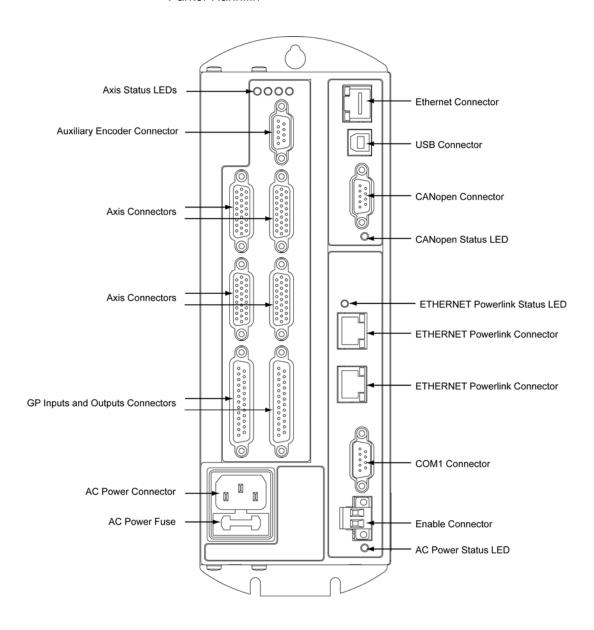
Figure 6 ACR9030 Front Panel Interfaces (2/4 Axis)
