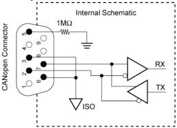
Figure 20 Equivalent Circuit for CANopen
