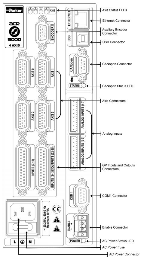
Figure 4 ACR9000 Stand-Alone Controller 2/4 Axis Front Panel Interfaces
