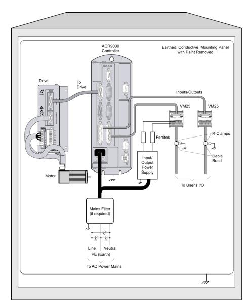
Figure 37 Typical LVD/EMC Installation
