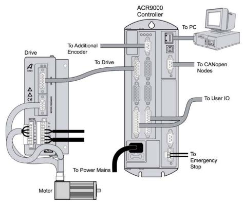
Figure 21 Overview of System Installation
