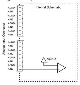
Figure 19 Equivalent Circuit for Single-Ended Analog Inputs
