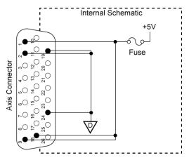
Figure 8 Equivalent Circuit for Axis Power Source
