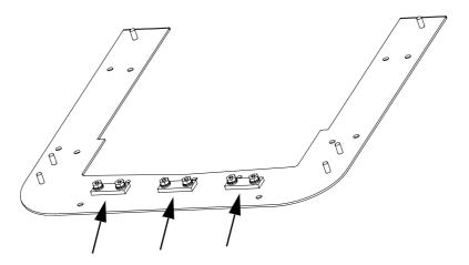
5. Slide the lower collar onto the drive module into the position shown. Fasten through the holes (arrowed) using the three screws removed at step 2.
