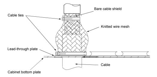
360° high frequency grounding of the control cable shields is recommended at their entries. The shields can be grounded by means of conductive shielding cushions pressed against the cable shield from both directions:
