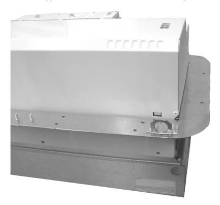
7. Attach the lateral supports to the drive module and the collars. Each support is fastened to the collars by four nuts, and to the drive module by three (out of six) screws removed at step 3.
