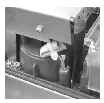
9. Near the top of the module, remove the grounding clip (held by two screws) that connects the varistor board to the module cover.
