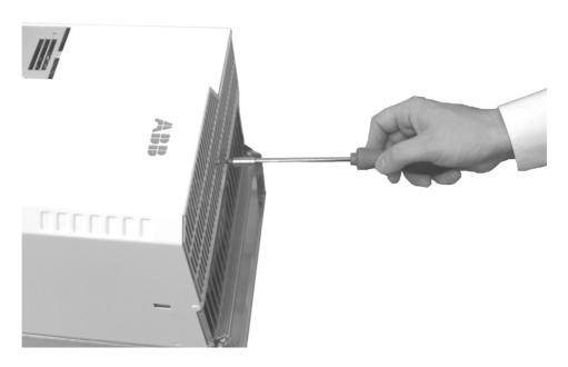
6. Remove the screws holding the drive module cover (8 on each side). Lift off the cover, bottom edge first.
