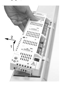
4. Disconnect the two cables coming to the mounting base of the JCU.
