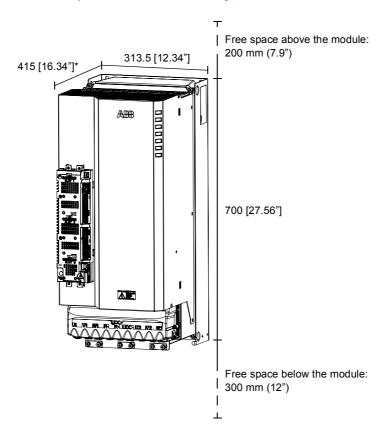
\*Including options installed on the JCU Control Unit. Note that the wiring to some option modules requires approximately 50 mm (2") of additional depth.
