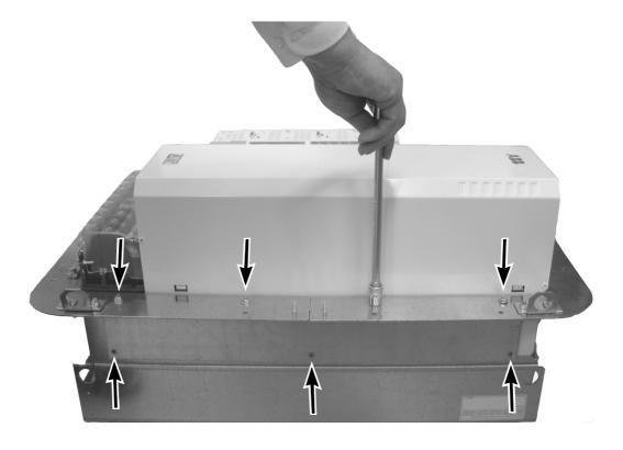
8. Join the collars by attaching lifting lugs on both sides. Attach further lifting lugs as needed.
