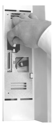
5. Remove the screw in the middle of the air outlet grating.
