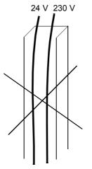
Not allowed unless the 24 V cable is insulated for 230 V or insulated with an insulation sleeving for 230 V.
