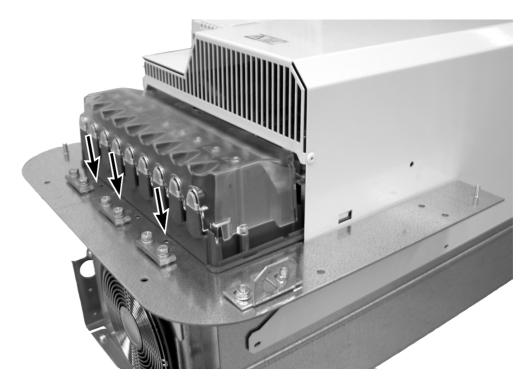
6. Slide the upper collar onto the drive module into the position shown.
