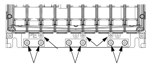
3. Remove the arrowed screws on each side of the module cover. (The middle row of screws is used later to attach the lateral supports of the mounting kit.)
