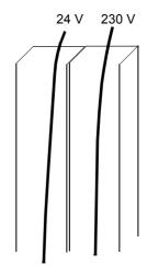
Lead 24 V and 230 V control cables in separate ducts inside the cabinet.
