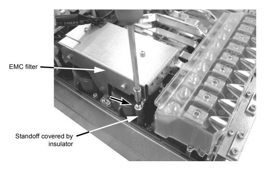
8. Insulate the end of the grounding wire reliably with insulating tape, tube sleeving and a cable tie.
