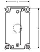
NOTES: 1. CATALOG DRAWING IS FOR REFERENCE ONLY 2. SEE ACTUAL PART DRAWING FOR SPECIFIC DESIGN 3. COVER OPTIONS: -BLANK- NO HOLES -BLANK- NO HOLES -1PB - (1) 30 mm DIA. HOLE -2PB - (2) 30 mm DIA. HOLE -1PB22 - (1) 22 mm DIA. HOLE -2PB22 - (2) 22 mm DIA. HOLES
