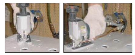
saw or fine toothed saw will provide the highest quality cutout with minimal edge chipping.
