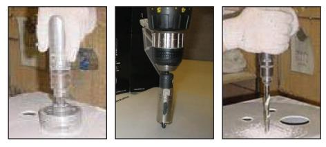
Using a drill with a positive rake angle and thin points or split points can help reduce cutting pressure. Feed rates must also be constant and may even be reduced upon exiting from a hole to reduce flexing of the part when the drill exits. Using a solid back surface to support the part when drilling can also aid in reducing delamination and chipping. Caution on polycarbonate to not generate enough heat that the material starts to melt or string.
