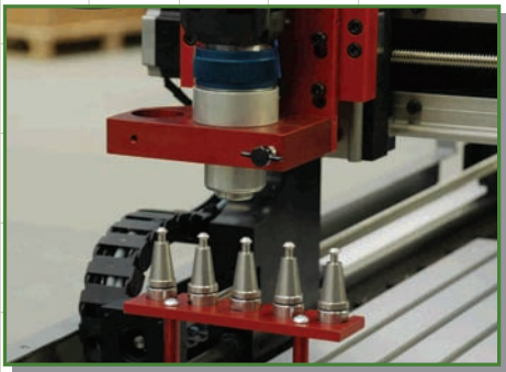
Optional 5 Station Automatic Tool Changer See Routing Accessories page 34.
