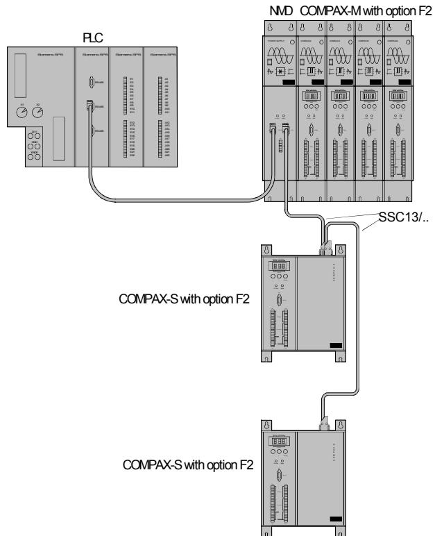
→ The Interbus-S signals are transferred along the existing ribbon cable within a COMPAX-M system network and a network module.
