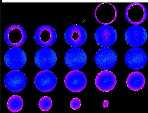
This result shows a PLG-405 laser pulse being stepped through a 4 ns gate window generated by a PHOTEK GM200-3N gate unit on a PHOTEK MCP118 image intensifier. Each step represents an extra 200 ps delay on the laser pulse.
