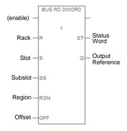
The rack and slot parameters identify which Memory Xchange module is to be accessed. The subslot should always be left blank or set to 0. The region parameter refers to one of the four memory regions in the Memory Xchange module. The offset is a 0 based number that specifies, in bytes, what portion of the memory region is to be accessed.
