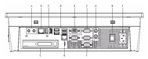
Figure 2.3 I/O Peripheral Connectors Panel of AC Input Model
