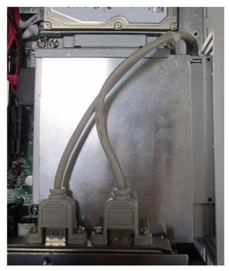
Figure 4.19 Dual-USB Cable Assembly on I/O Bracket
