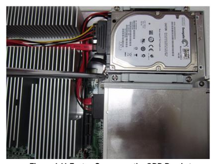
Figure 4.11 Fasten Screws on the ODD Bracket
