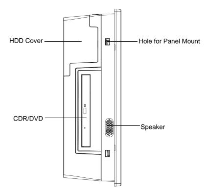
Figure 2.2 Side View of the Panel PC
