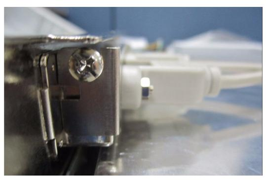
Figure 4.20 Fasten Screw on Bracket
