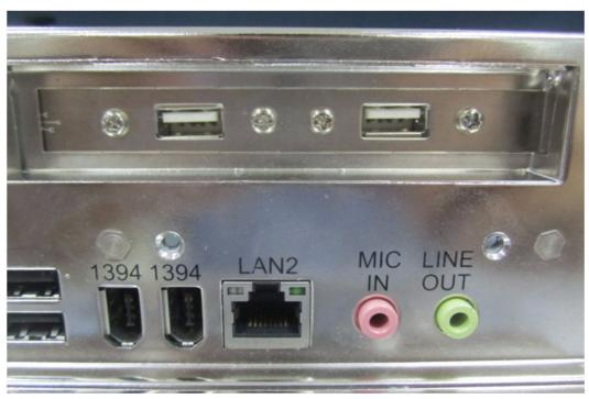
Figure 4.21 Completed Assembled Dual-USB Cable
