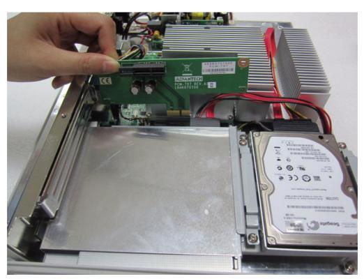
Figure 3.2 PCI & PCIe Bus Expansion
