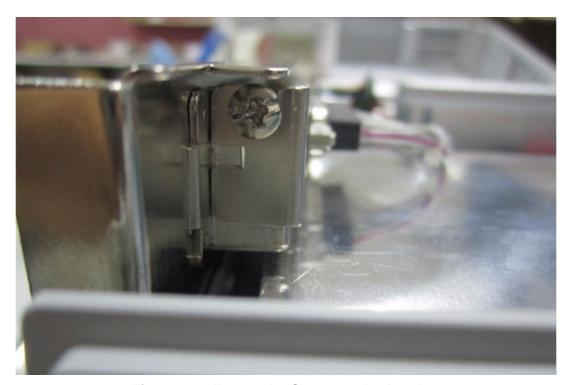
Figure 4.16 Fasten the Screw on the Bracket
