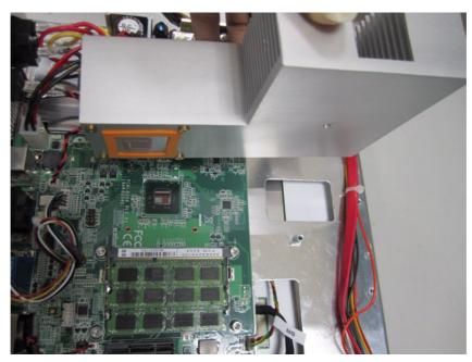
Figure 4.5 Placing the Memory Module in the SODIMM Socket
