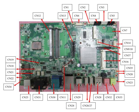
Figure 5.1 Jumpers & Connectors on PPC-L158T Motherboard
