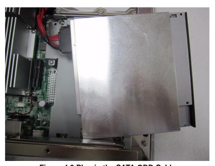
Figure 4.9 Plug in the SATA ODD Cable
