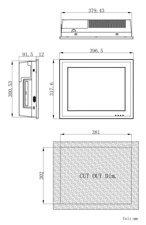
Figure 1.1 Dimensions of PPC-L158T
