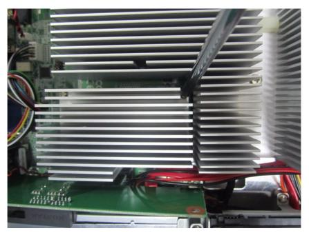
Figure 4.7 Fasten the Memory Heatsink onto the Board
