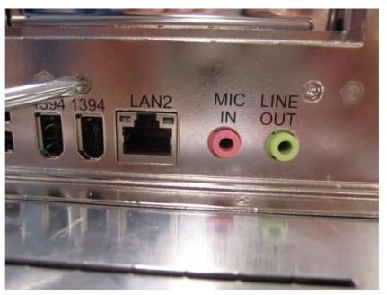
Figure 4.10 Fasten Screw on IO Shielding
