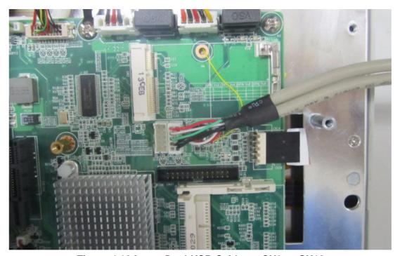
Figure 4.18 Insert Dual-USB Cable on CN9 or CN10
