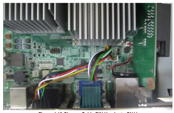
Figure 4.13 Change Cable PIN Header to CN11
