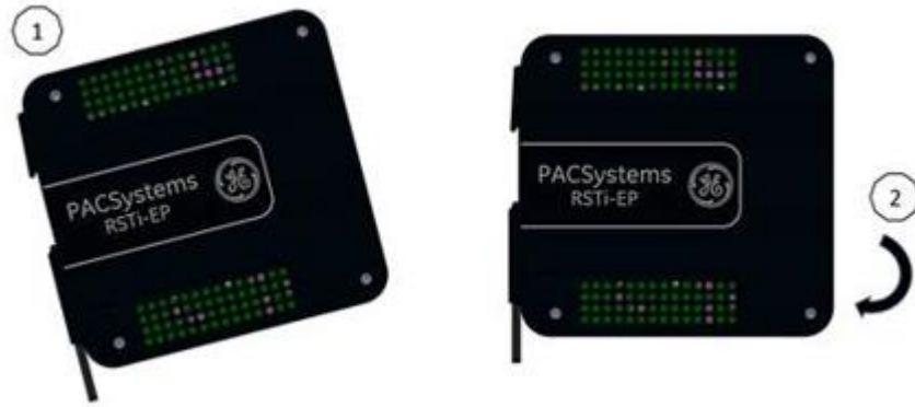
Figure xx: Mounting positions of the EPSCPE100 on DIN rail
