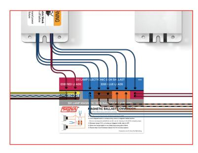
Make sure you are ready for the conversion. Wiring blocks are available for 4, 5, and 6 lamp installations using either four or six lamp ballasts.
