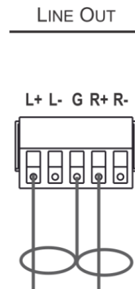
Figure 6: Connecting to an Unbalanced Stereo Audio Acceptor
