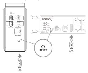
The "RESET" button is located on the front panel of rackmount type switches and on the top panel of DIN-rail type switches.
