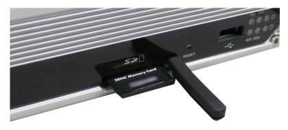
**Step 3:** Gently move the protective cover back to the SD slot. Power on the embedded computer and start the operating system.
