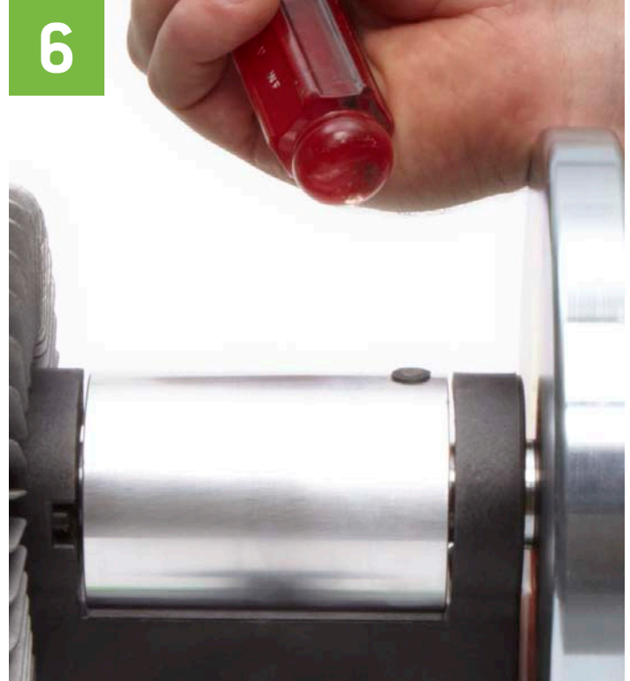
6 Magnet should be flush with top of grommet
