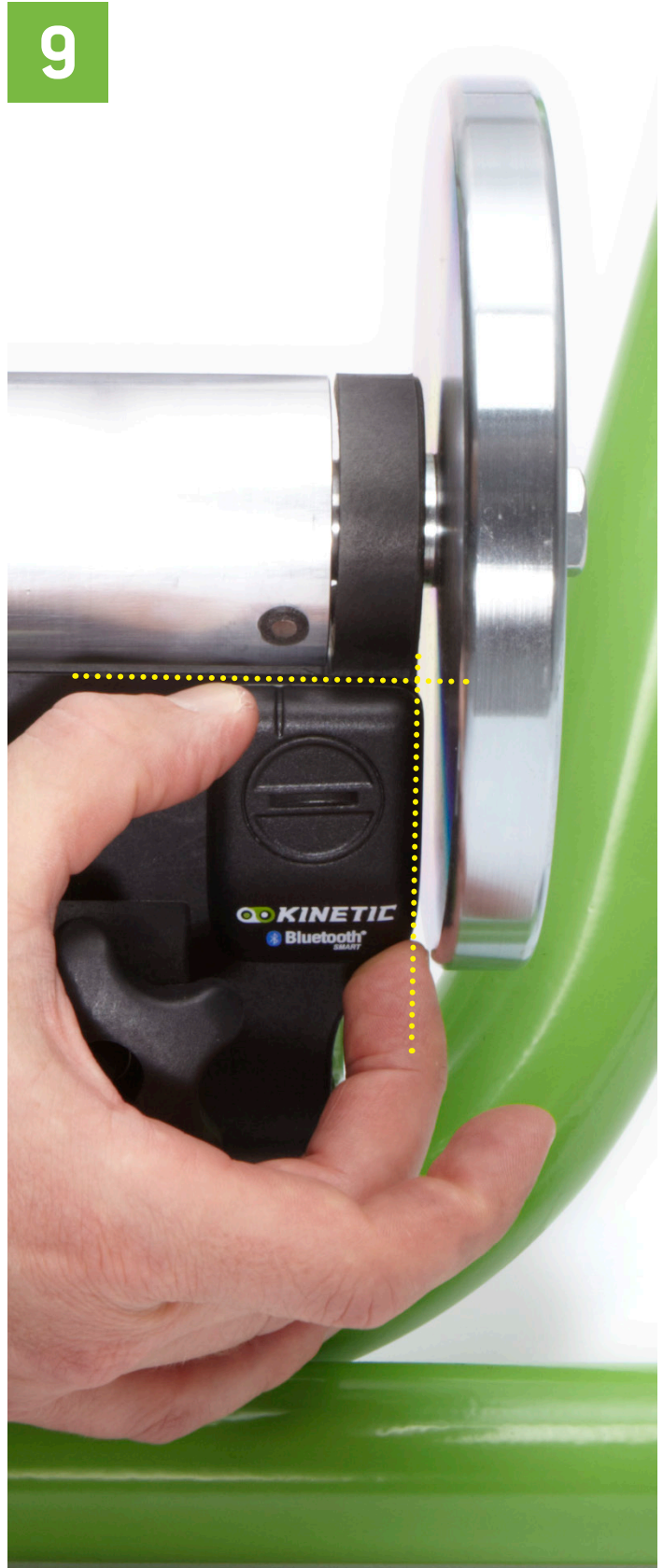
Carefully position and place sensor on trainer yoke bracket and press into place. NOTE: alignment is critical. Edges of sensor must match edges of trainer yoke bracket.
