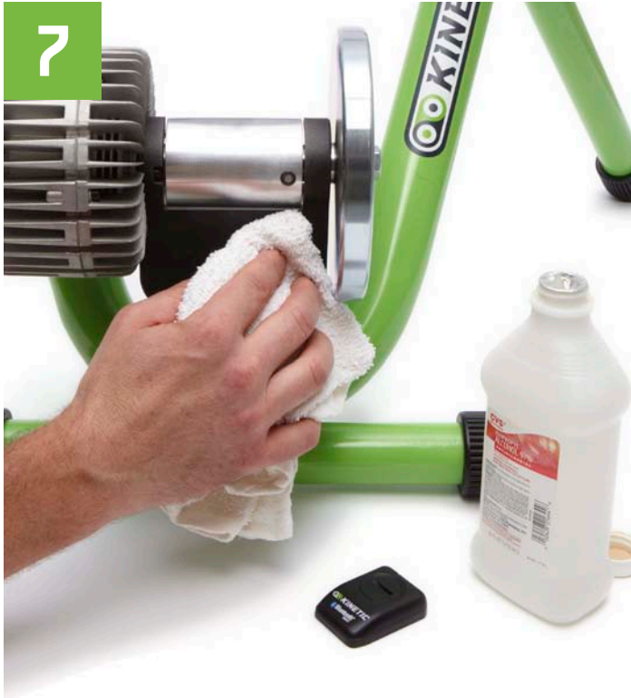
Clean plastic surface with isopropyl alcohol
