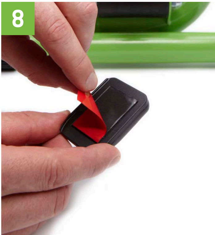
Peel backing from adhesive patch on sensor
