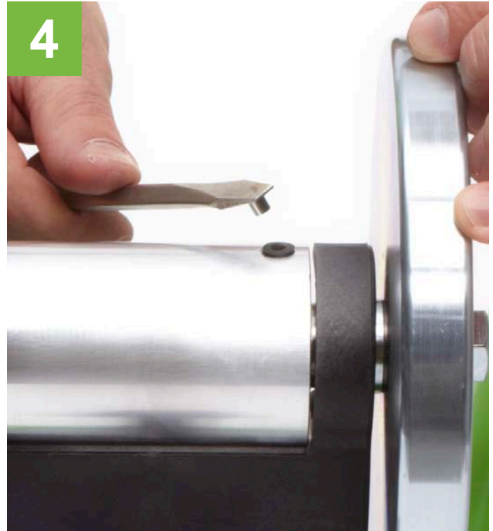
4 Using screwdriver, press magnet into grommet
