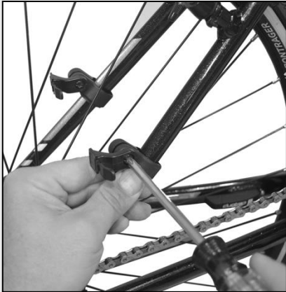
Step 1. Placement of Lights in TSC Install the seat-stay brackets anywhere below the brakes. They should be level with each other.
