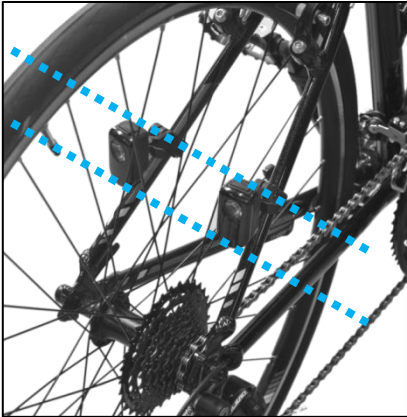
Step 2. After attaching the lights, make sure the lights are level with each other in relation to the ground plane.
