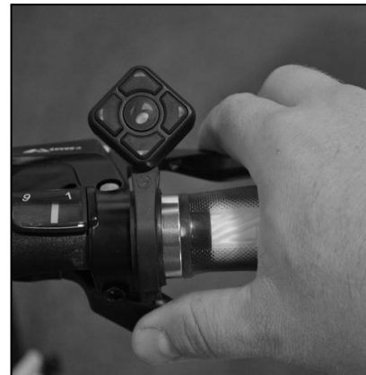
In front of the bar between the shifter and the grip (flat bars) Note: placement of the remote will depend on personal preference and clearance with shift levers.
