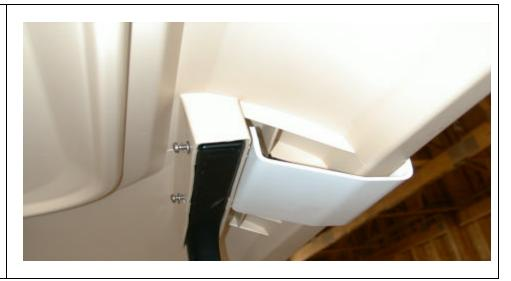
3. Attach Antenna bracket with screws and lock tight.
