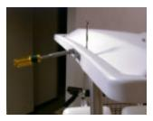
Mount UHF antenna on right side of cart using the two Phillips head screws, flat washer and sheathing pieces.
