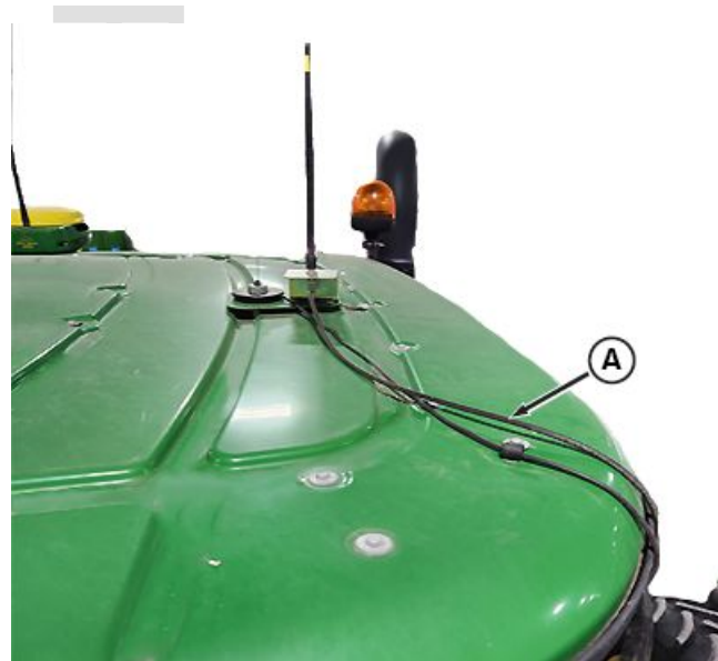
Route Antenna Cable—Cab Roof
