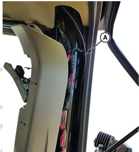
Antenna Cable Routing
