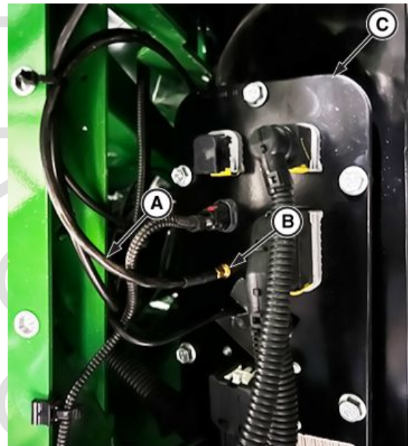
Antenna Cable Connection
