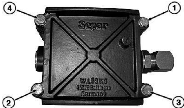
Lid Cap Screw Tightening Sequence
