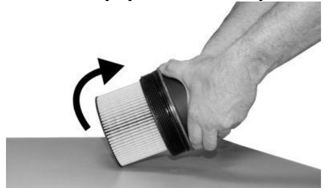
Removing Engine Oil Filter From Cover
