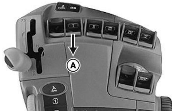
SCV Control Lever Extend and Extend Detent
