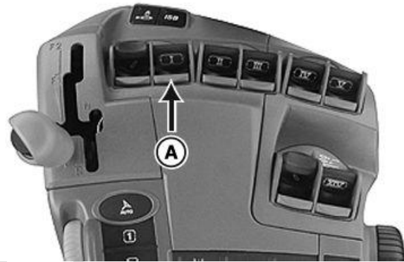
SCV Control Lever Retract and Retract Detent
