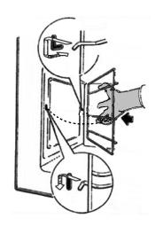
To remove the side racks, lift and pull out the front, slide the rack forwards and lift free.
