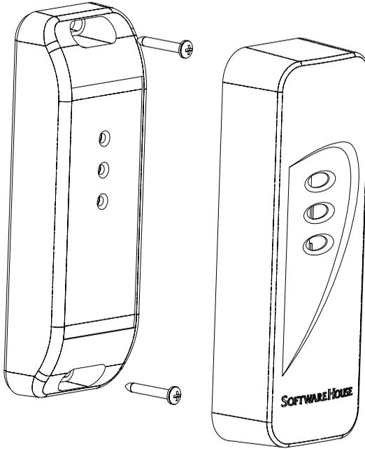
FIGURE 1. Mounting Assembly
