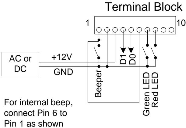
FIGURE 2. Beeper Wiring
