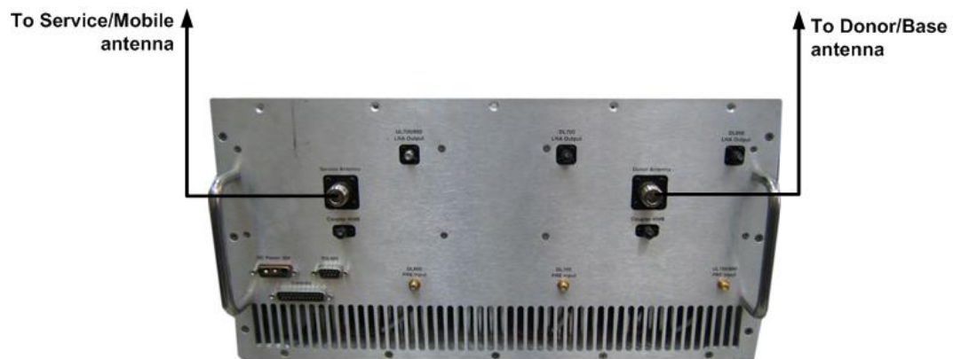
Figure 8. Power Amplifier and Antenna Connections
