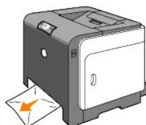
4. Open the front cover by pushing the button (right side) and remove the jammed paper. Then, confirm that there are no scraps of paper remaining inside the printer.
