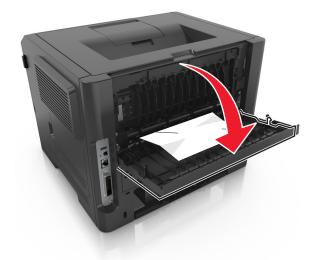
**3** Firmly grasp the jammed paper on each side, and then gently pull it out. **Note:** Make sure all paper fragments are removed.
