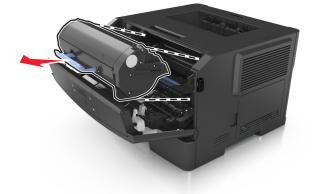
**3** Lift the blue handle, and then pull the imaging unit out of the printer.
