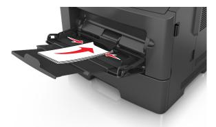
**Warning—Potential Damage:** Never use envelopes with stamps, clasps, snaps, windows, coated linings, or self-stick adhesives. These envelopes may severely damage the printer.
