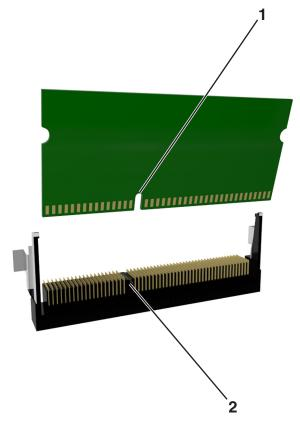
**4** Push the memory card straight into the connector, and then push the card toward the controller board wall until it *clicks* into place.
