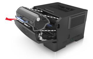
**3** Lift the blue handle, and then pull out the imaging unit from the printer.
