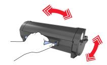
**5** Insert the toner cartridge into the printer by aligning the side rails of the cartridge with the arrows on the side rails inside the printer.
