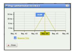
Select this option from the Direct Access menu to initiate ICMP ping, and to display a progress bar, and graph of the selected device's ping responses.
