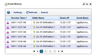
The initial portlet view displays an icon whose color reflects any alarm state associated with the event. It also displays the *Receive Time*, *Entity Name*, *Device IP*, and *Event Name*. You can right-click to *Share with User* in this screen.
