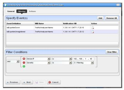
Click *Add Filter* to further filter the selected events. See Filter Expanded Portlet Displays on page 85 for more about this feature. After you *Add Filter* the button changes to *Clear Filter* so you can remove any filter from the event rule.
