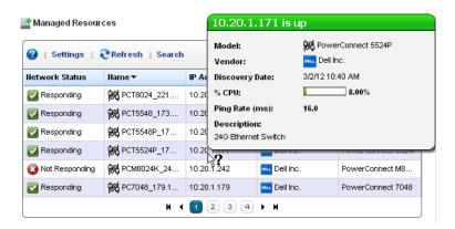
Hovering the cursor over a listed device's IP address produces a popup with its alarm status in the headline (both severity name and color), the % CPU, % Memory, and Ping. See the Managed Resources Expanded section for a description of columns and additional capabilities in that version of the portlet. Icons that appear next to the equipment name have some significance. For example:
