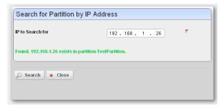
Clicking Search locates the mediation partition that services the entered IP address (although it does not determine whether that partition is up and running).
