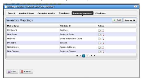
You can Add a new mapping with that button, or Remove All listed mappings with that button. You can also edit or delete listed mappings with the Action icons to the right of each row. Adding or editing opens the Inventory Mapping Editor.
