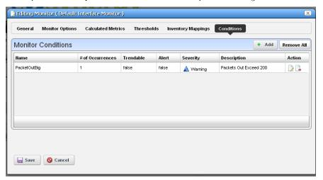
Click the Add button to enter a new set of conditions, or click the Edit this entry button to the right of a listed Monitor Condition to open the editor. Click the Delete button to remove a listed set of conditions. Click the Copy icon to duplicate the listed condition.
