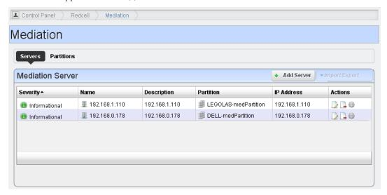
Mediation server, routing entries and partition entries appear automatically when mediation server connects for the first time. You can test connectivity from appserver cluster and medserver/partition.
