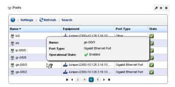
This displays a list of ports, with columns for *Port Icon, Equipment Name*, *Name*, *Type* and *Encapsulation*. Hover your cursor over the *Name* column, and a popup appears adding the port's *Date Created* and *Operational State* information. Right-clicking offers a subset of the actions listed in Managed Resources on page 166. You can also create links. See Ports > Links on page 182. See Port Editor on page 194 for details of the editor specifically for ports.
