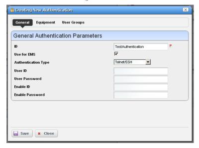
The fields that appear in this editor vary, depending on the type of authentication. The *ID* (name) for the authentication is mandatory. If you *Add* an existing authentication, for example to Discovery Profiles, you can also configure the Management Interface Parameters like *Timeout*, *Retries*, and *Port* used. If you have an authentication that works for multiple protocols (for example SSH or Telnet), you can also select the *Protocol Type*.
