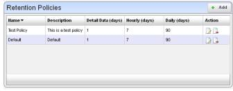
All monitors rely on a polling engine which provides runtime mediation activities for distributed device interaction at regular intervals. Monitors may share a retention policy. Data is rolled up hourly and daily into summary data. The retention policy controls how long data is held per roll-up period.
