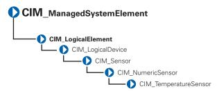
The CIM\_TemperatureSensor class described in Table 3-10 contains sensors that sample ambient temperature and return a value in degrees celsius.
