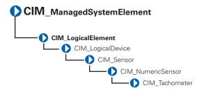
The CIM\_Tachometer class described in Table 3-13 contains devices that measure revolutions per minute (RPM) of a fan and return the value in RPMs.
