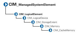
The CIM\_CacheMemory class described in Table 3-30 describes the capabilities and management of cache memory. Cache memory allows a microprocessor to access data and instructions faster than normal system memory.
