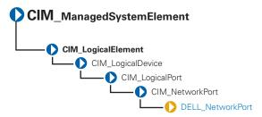
The Dell\_Network Port class described in Table 4-12 represents the Dell-specific features of the network adapters.
