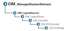
The CIM\_PCIBridge class described in Table 3-26 describes the capabilities and management of a PCI controller providing bridge-to-bridge capability. An example is a PCI to Industry-Standard Architecture (ISA) bus bridge.
