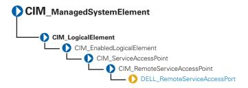
The DELL\_RemoteServiceAccessPort class described in Table 3-46 is an extended class of the CIM\_RemoteServiceAccessPoint class. The DELL\_RemoteServiceAccessPort class provides information about Dell implementation-specific attributes.
