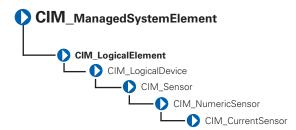
The CIM\_Sensor class described in Table 3-7 contains hardware devices capable of measuring the characteristics of some physical property, for example, the temperature or voltage characteristics of a computer system.
