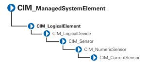
The CIM\_CurrentSensor class described in Table 3-11 contains sensors that measure amperage and return a value in amperes and watts.
