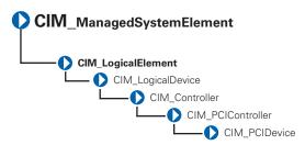
The CIM\_PCIDevice class described in Table 3-25 describes the capabilities and management of a PCI device controller on an adapter card.
