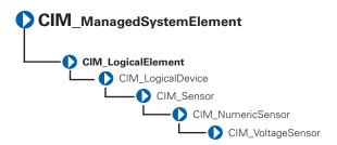
The CIM\_VoltageSensor class described in Table 3-12 contains sensors that measure voltage and return a value in volts.
