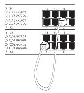
Each port supports Auto MDI & MDI-X functionality. When cascading with other switches or hubs, each port can connect directly to a switch or hub with straight through twisted pair cable.
