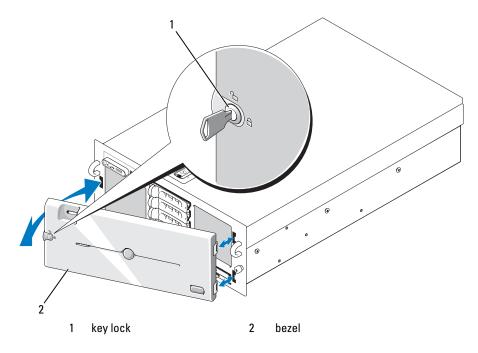
To replace the optional bezel, hook the right end of the bezel onto the chassis, then fit the free end of the bezel onto the system. Secure the bezel with the keylock. See Figure 3-2.
