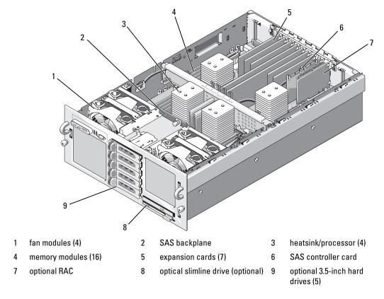
The system board holds the system's control circuitry and other electronic components. The processors and memory modules are installed directly on the system board.
