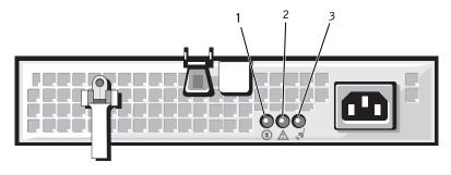
AC line status indicator power supply status indicator power supply fault indicator
