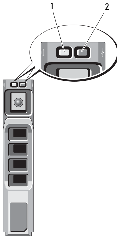
Figure 1-3. Hard Drive Indicators
