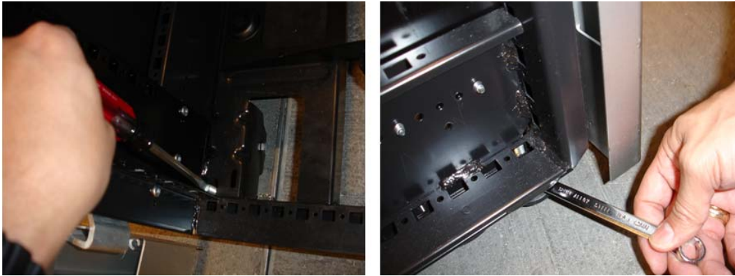
Figure 6: Leveling Feet Deployment
