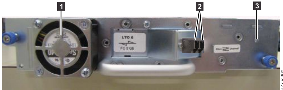
Figure 1-3. Rear panel (drive sled only) of a half height Fibre Channel drive
