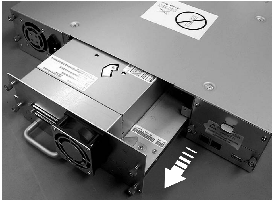
Figure 10-16. Removing a drive sled from the library (drive sled without ESD springs shown)
