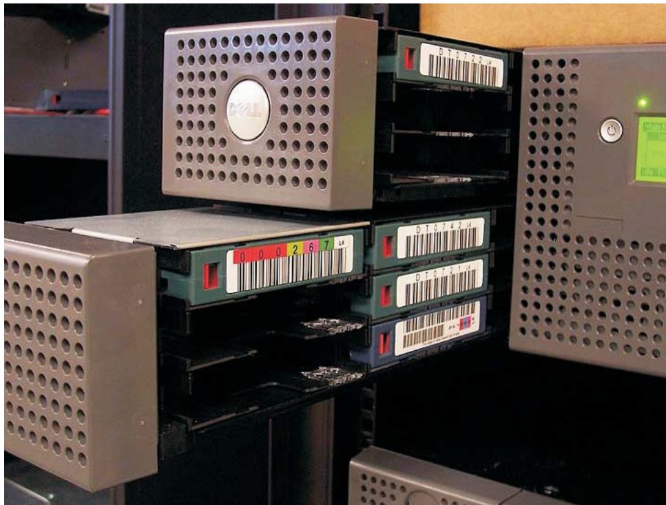
Figure 4-44. 4U library I/O station in the lower left magazine
