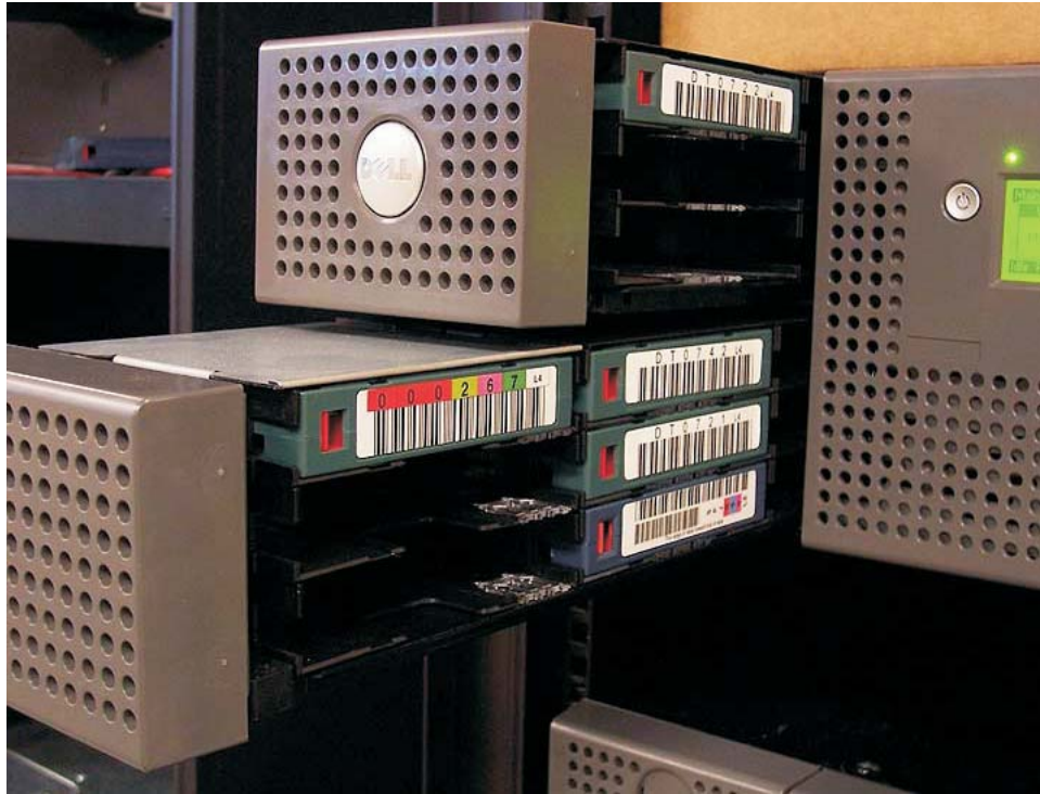
Figure 10-23. Left magazines pulled out of a 4U library (facing front of library)
