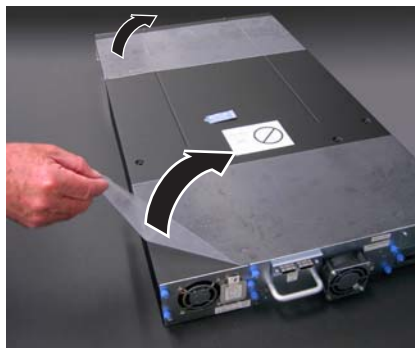
Figure 4-1. Removing the plastic protective sheets from the library
