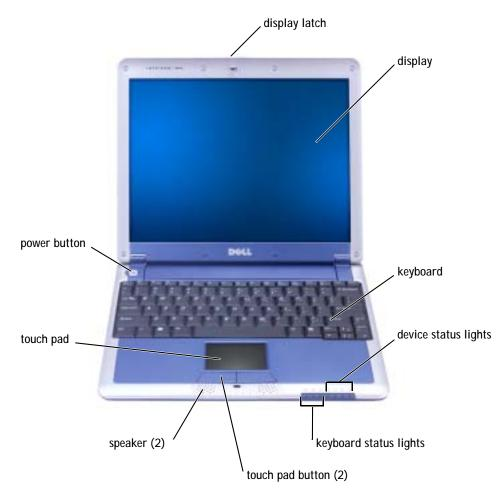
**DISPLAY LATCH** — Keeps the display closed.
