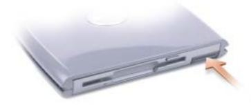
2 Pull the device by the latch release to remove the device from the D/Bay.
