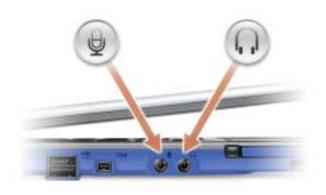
Attach a microphone to the  $\Theta$  connector.
