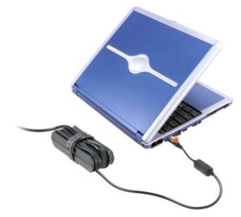
CAUTION: If you are using a multiple-outlet power strip, use caution when plugging the AC adapter's power cable into the power strip. Some power strips may allow you to insert the plug incorrectly. Incorrect insertion of the power plug could result in permanent damage to your computer, as well as risk of electric shock and/or fire. Ensure that the ground prong of the power plug is inserted into the mating ground contact of the power strip.
