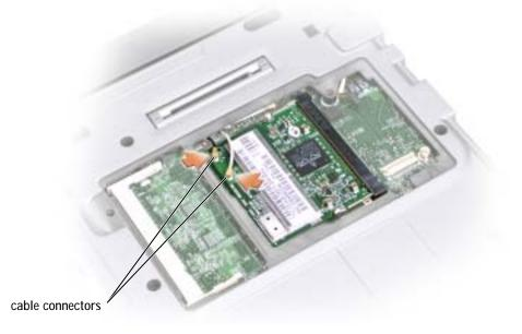
**b** Release the Mini PCI card by spreading the metal securing tabs until the card pops up slightly.
