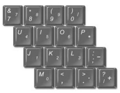
The numeric keypad functions like the numeric keypad on an external keyboard. Each key on the keypad has multiple functions.
