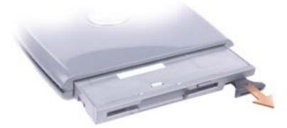
5 Insert the new device into the bay, push the device until it clicks, and push the device latch release in so that it is flush with the bay.
