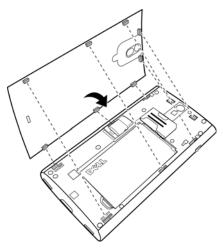
**b** Place the cover onto the back of the smartphone, and then slide the cover towards the top of the smartphone to secure the cover in place.
