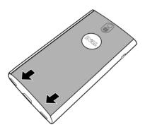
**b** Lift the back cover off the smartphone.
