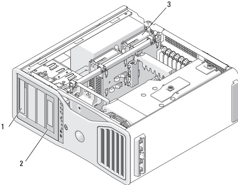
1 four 5.25-inch drive bays (can hold an optical drive, floppy drive, Media Card Reader, or SATA hard drive in a special drive case)
