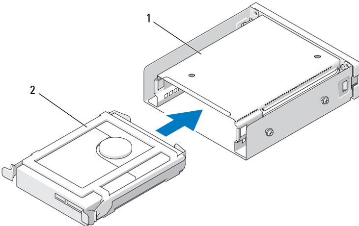
1 hard-drive carrier      2 hard drive in hard-drive bracket
