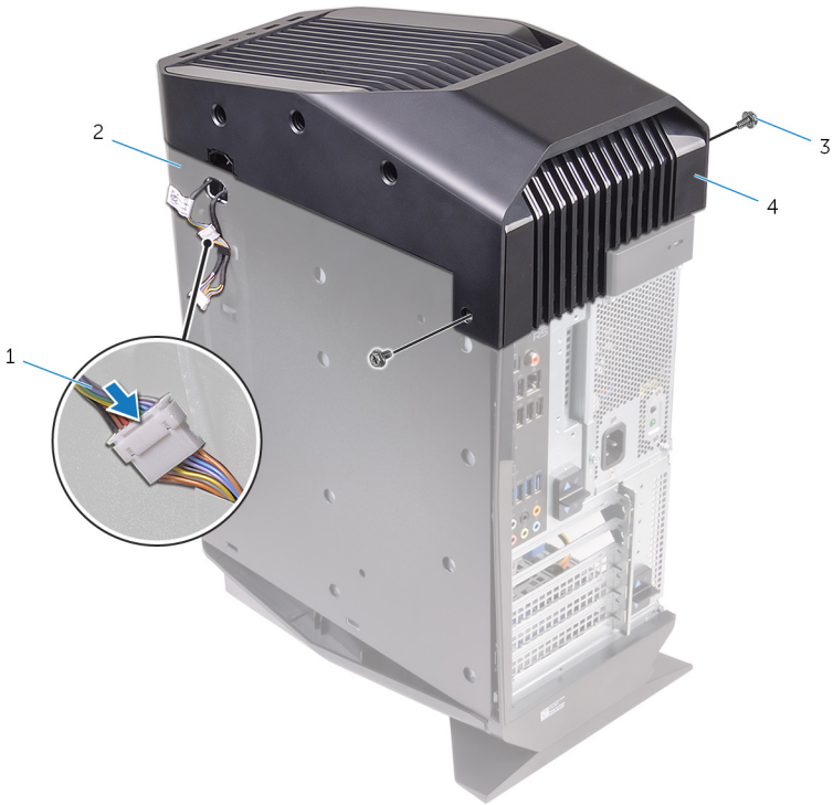
Figure 15. Replacing the top cover
