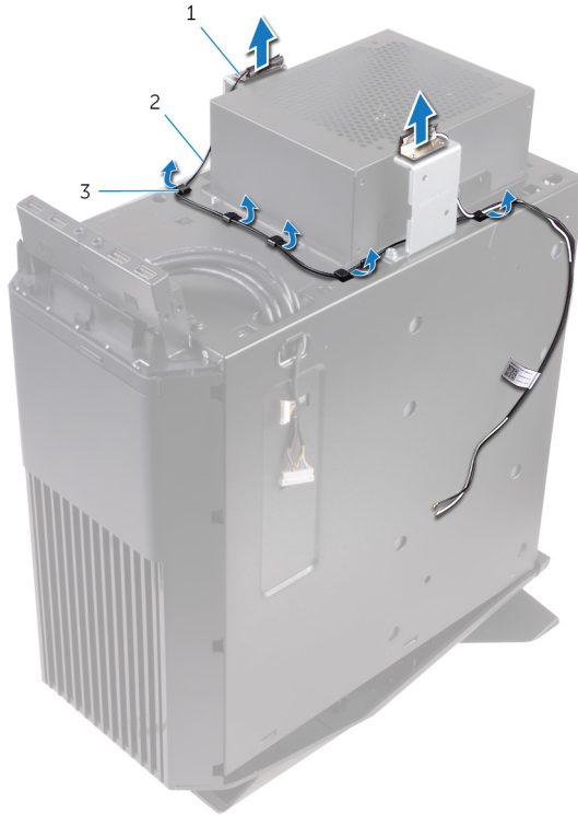
Figure 36. Removing the antenna cables
