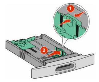
**3** Unlock the length guide, squeeze the length guide tab inward as shown, and slide the guide to the correct position for the paper size being loaded.
