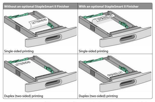
**Note:** Notice the maximum fill line on the side of the tray which indicates the maximum height for loading paper. Do not overload the tray.
