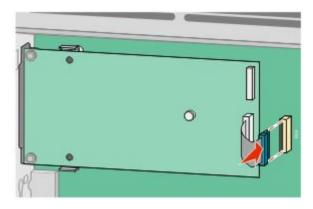
**12** If a printer hard disk was previously installed, then attach the printer hard disk to the ISP. For more information, see "Installing a printer hard disk" on page 28.
