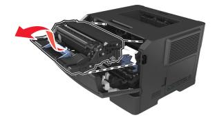
**Warning—Potential Damage:** Do not touch the shiny blue photoconductor drum under the imaging unit. Doing so may affect the quality of future print jobs.
