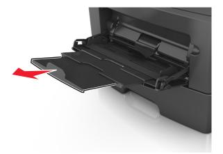
**b** Pull the extender gently so that the multipurpose feeder is fully extended and open.
