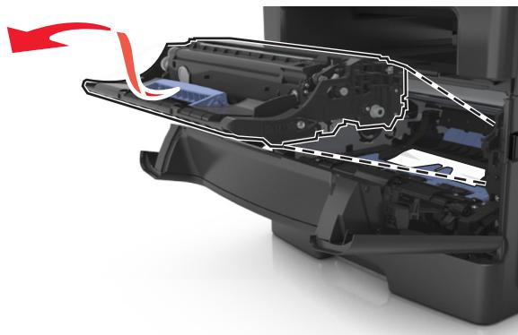
**Warning—Potential Damage:** Do not touch the shiny blue photoconductor drum under the imaging unit. Doing so may affect the quality of future print jobs.
