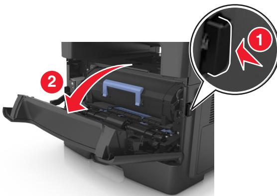
**2** Pull the toner cartridge out using the handle.
