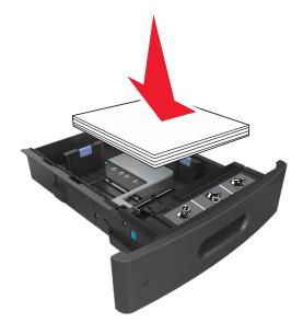
• Make sure the guides in the tray or the multipurpose feeder are properly positioned and are not pressing tightly against the paper or envelopes.
