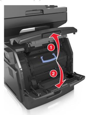
**2** Pull out the toner cartridge from the printer using the handle.
