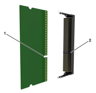
**4** Push the memory card straight into the connector, and then push the card toward the controller board wall until it *clicks* into place.
