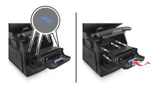
7 Insert the toner cartridge into the printer by aligning the side rails of the cartridge with the arrows on the side rails inside the printer.
