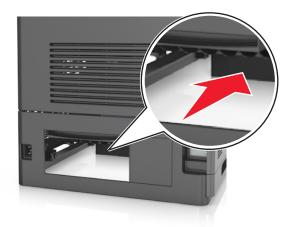
**5** Press down the rear duplex flap, then firmly grasp the jammed paper, and then gently pull the paper out. **Note:** Make sure all paper fragments are removed.
