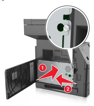
Tighten the screws on the shield.
