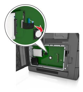
**3** Remove the screws holding the printer hard disk in place.
