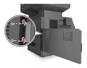
4 Remove the printer hard disk.
