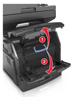
**2** Lift the blue handle, and then pull out the toner cartridge from the printer.
