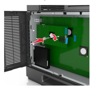
**Note:** Turn the screw clockwise, enough to hold the ISP in place, but do not tighten it yet.
