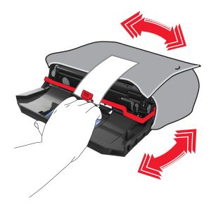
**5** Remove all packing material from the imaging unit.
