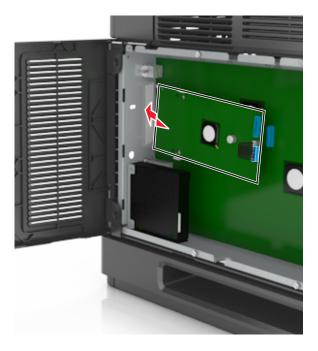
**Note:** Hold the ISP at an angle over the plastic bracket so that any overhanging connectors will pass through the ISP opening in the cage.
