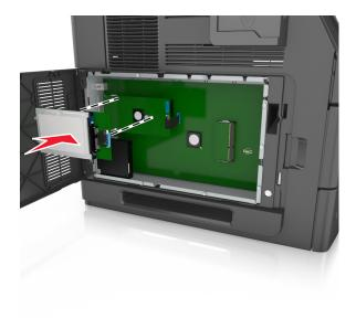
**c** Insert the plug of the printer hard disk interface cable into the receptacle of the ISP.
