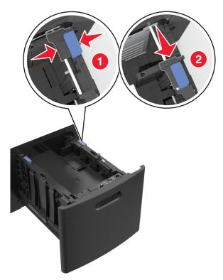
**c** Remove the A5 length guide from its holder.
