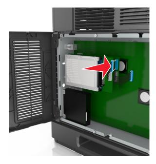
To install a printer hard disk directly on the controller board cage:
