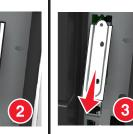
**5** Align the posts of the plastic bracket to the holes on the controller board cage, and then press the plastic bracket on the controller board cage until it *clicks* into place.
