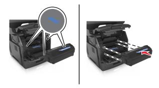
**Warning—Potential Damage:** When replacing a toner cartridge, do not leave the imaging unit exposed to direct light for an extended period of time. Extended exposure to light may cause print quality problems.
