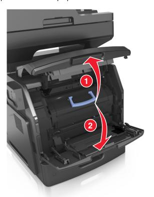
**2** Pull the cartridge out of the printer using the handle.
