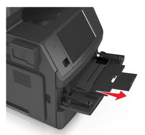
**Note:** Guide the extender gently so that the multipurpose feeder is fully extended and open.
