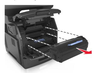
**3** Lift the blue handle, and then pull out the imaging unit from the printer.
