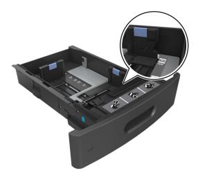
**3** Unlock the length guide, and then squeeze and slide the guide to the correct position for the size of the paper you are loading.
