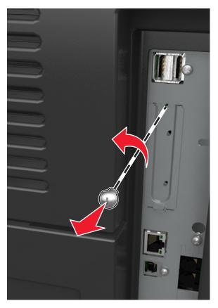
**b** Lift the metal cover, and then pull it out completely.
