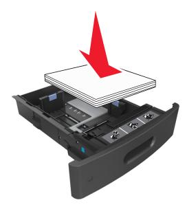
• If you are loading envelopes, then make sure that the flap side is facing up and the envelopes are on the left side of the tray.
